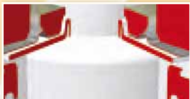
T4E with additional metal diaphragm
